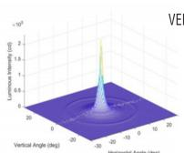
LED COMPETITOR - COMPLIANT BUT VERY THIN BEAM PATTERN / DOES NOT FLOOD THE AREA
